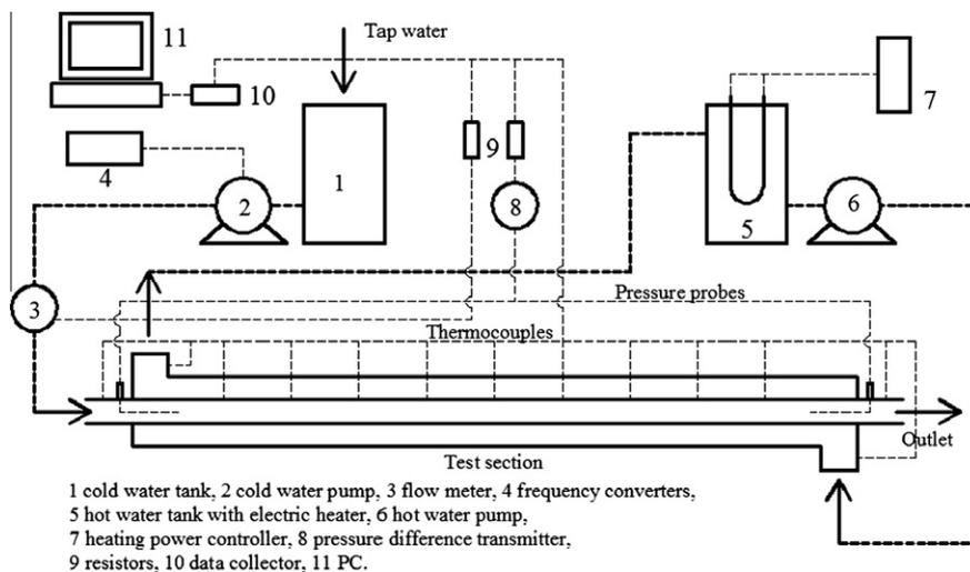
1 cold water tank, 2 cold water pump, 3 flow meter, 4 frequency converters, 5 hot water tank with electric heater, 6 hot water pump, 7 heating power controller, 8 pressure difference transmitter, 9 resistors, 10 data collector, 11 PC.
