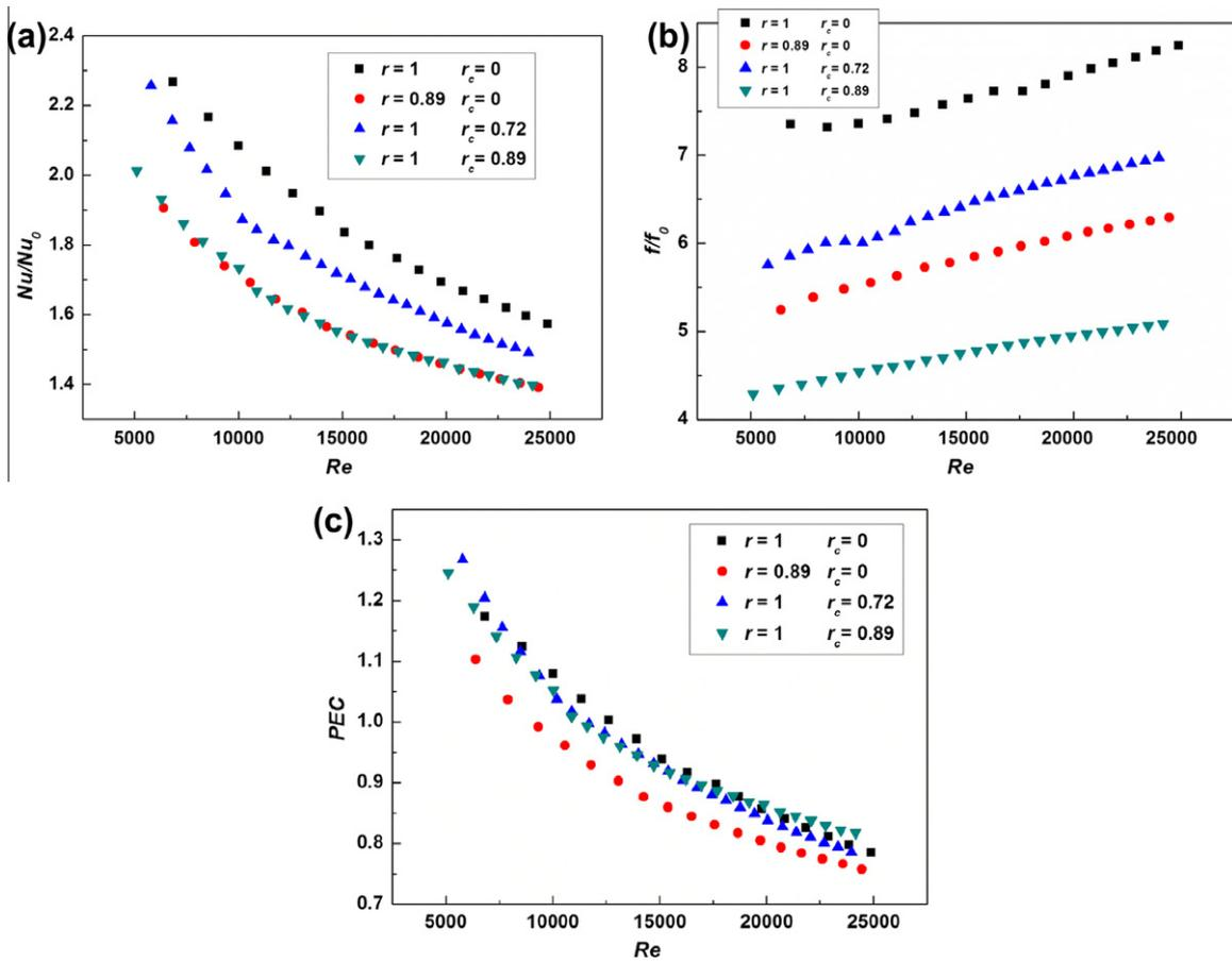
**Fig. 7.** The Nusselt number ratio ( $Nu/Nu_0$ ), the friction factor ratio ( $f/f_0$ ) and the thermal performance factor ( $PEC$ ) versus the Reynolds number ( $Re$ ) for conical-strip inserts with different upwind areas: (a)  $Nu/Nu_0$ , (b)  $f/f_0$ , and (c)  $PEC$ .
