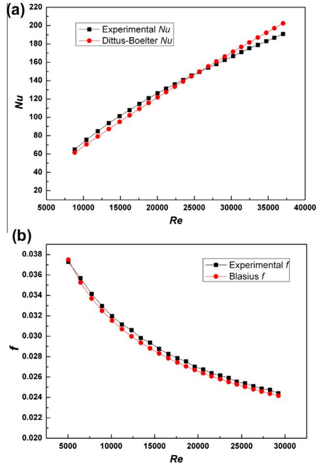
Fig. 5. The Nusselt number ( $Nu$ ) and friction factor ( $f$ ) versus the Reynolds number ( $Re$ ) for turbulent flow in smooth: (a)  $Nu$  and (b)  $f$ .
