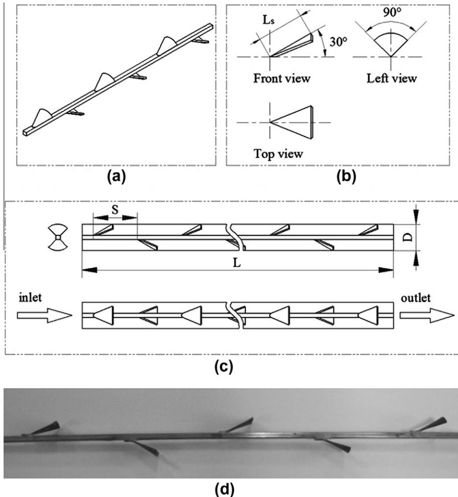
Fig. 1. (a) Schematic of the conical-strip insert, (b) geometry of the conical strip, (c) schematic of the circular tube with the conical-strip insert, and (d) picture of the conical-strip insert.
