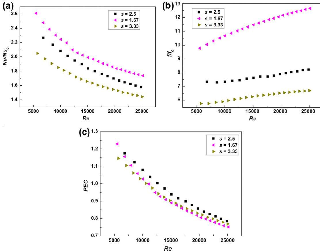
Fig. 8. The Nusselt number ratio ( $Nu/Nu_0$ ), the friction factor ratio ( $ff/f_0$ ) and the thermal performance factor ( $PEC$ ) versus the Reynolds number ( $Re$ ) for conical-strip inserts with different pitches: (a)  $Nu/Nu_0$ , (b)  $ff/f_0$ , and (c)  $PEC$ .
