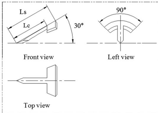
Fig. 3. Geometry of the T-type conical strip.
