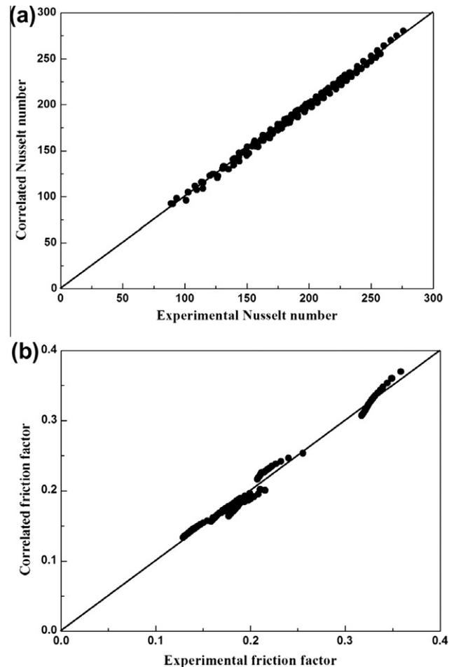
Fig. 9. Comparison of experimental results with the correlated values: (a)  $Nu$  and (b)  $f$ .
