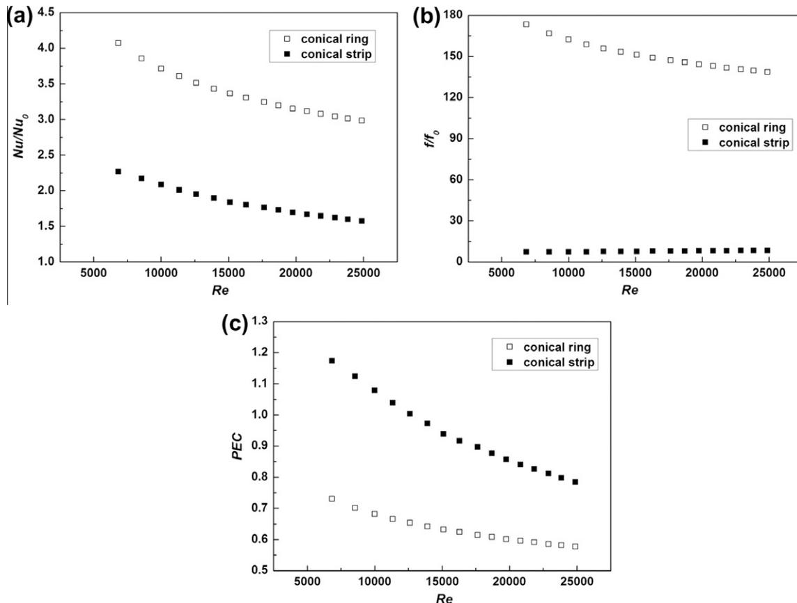
Fig. 6. Comparisons of the Nusselt number ratio ( $Nu/Nu_0$ ), the friction factor ratio ( $ff/fo$ ) and the thermal performance factor (PEC) for the conical-strip and conical-ring inserts: (a)  $Nu/Nu_0$ , (b)  $ff/fo$ , and (c) PEC.
