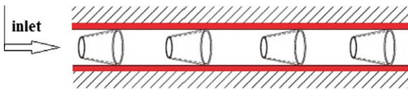
Fig. 2. Sketch of the tube with conical rings.
