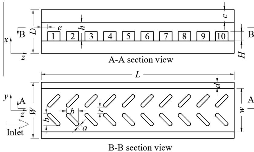
Fig. 1. Schematic view of the mini-channel with discrete double-inclined ribs.
