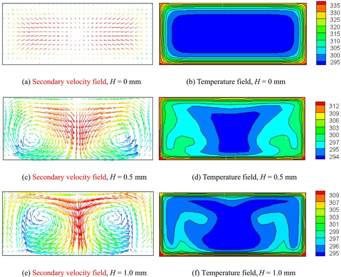
Fig. 3. Tangential velocity and temperature fields at the cross-section ( $z/L = 0.5$ ),  $Re = 600$ .
