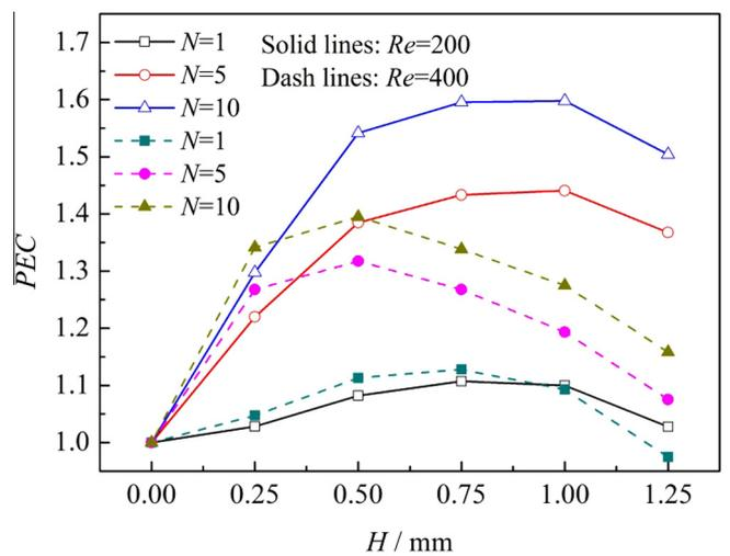
Fig. 9. Comparison of  $PEC$  values under different ribs numbers.
