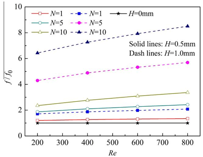
Fig. 8. Variations of the flow performance under various ribs numbers with Reynolds number.
