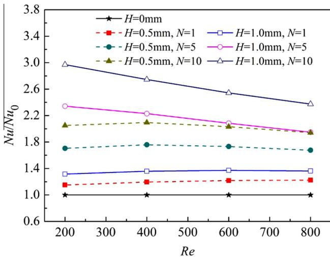
Fig. 6. Variations of the heat transfer performance under various ribs numbers with Reynolds number.
