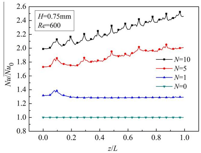
Fig. 7. Variations of average  $Nu/Nu_0$  under different ribs numbers along the flow direction.
