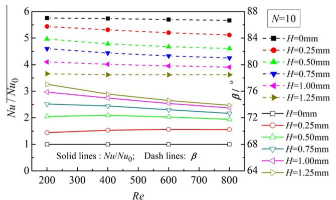
Fig. 2. Variation of the heat transfer and field synergy performance under various ribs heights with Reynolds number,  $N = 10$ .
