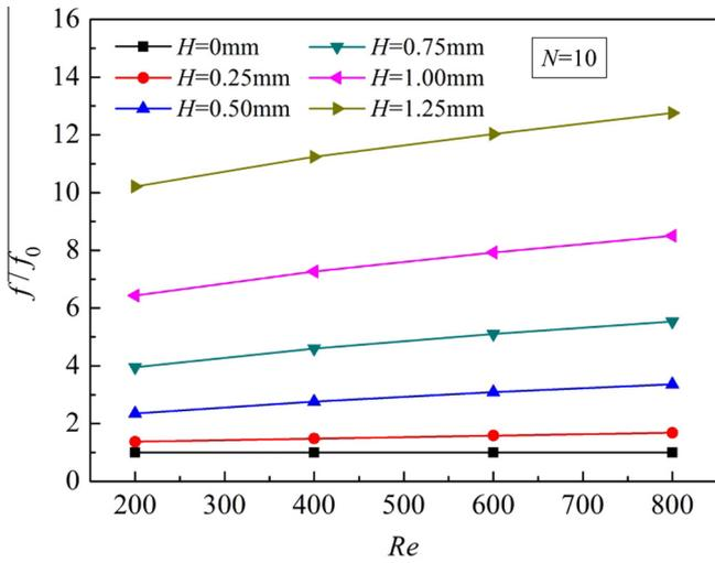
Fig. 4. Variations of the flow performance under various ribs heights with Reynolds number,  $N = 10$ .
