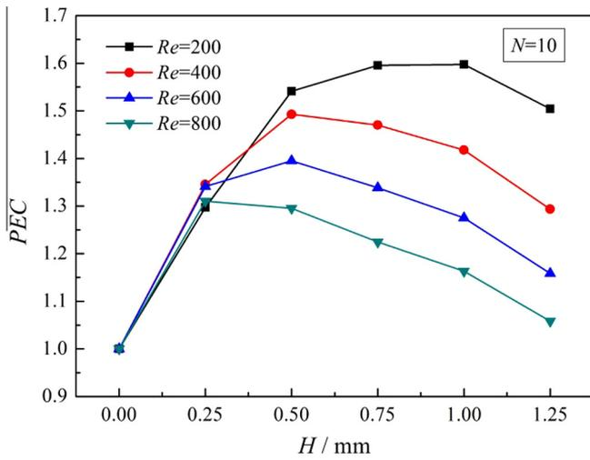
Fig. 5. Variations of the  $PEC$  under different Reynolds numbers with ribs height,  $N = 10$ .
