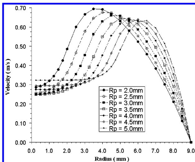
7 Influence of porous medium packing radius on inner tube velocity profiles
