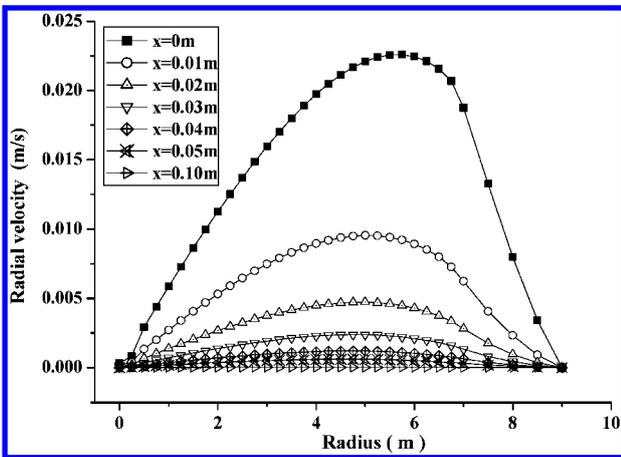
4 Radial velocity profiles when  $R_p$  is 7 mm and Re number is 250
