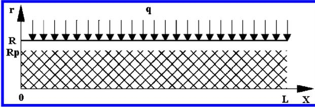
1 Model of tube filled with metal porous medium in central area
