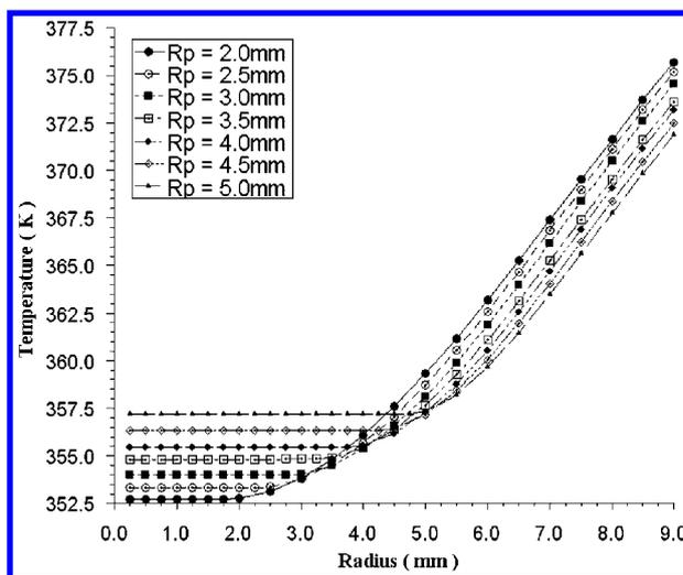
8 Influence of porous medium packing radius on inner tube temperature profiles
