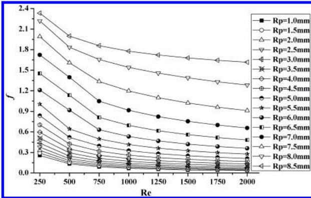
9 Influence of porous medium packing radius and Re number on resistance coefficient  $f$
