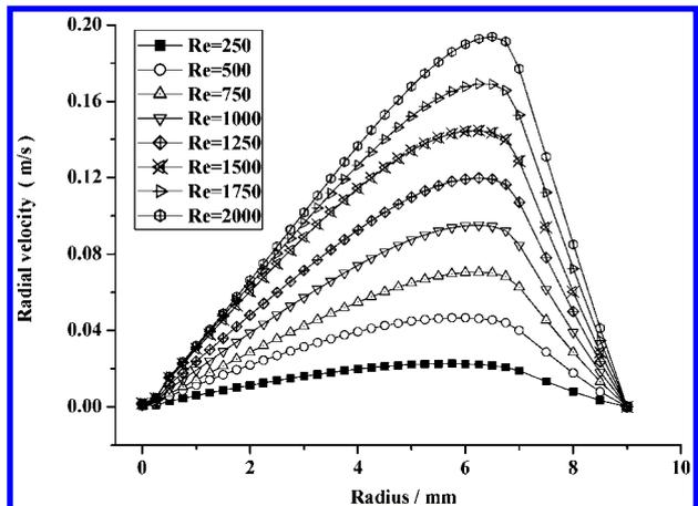
5 Inlet radial velocity profiles under different Re numbers when  $R_p$  is 7 mm
