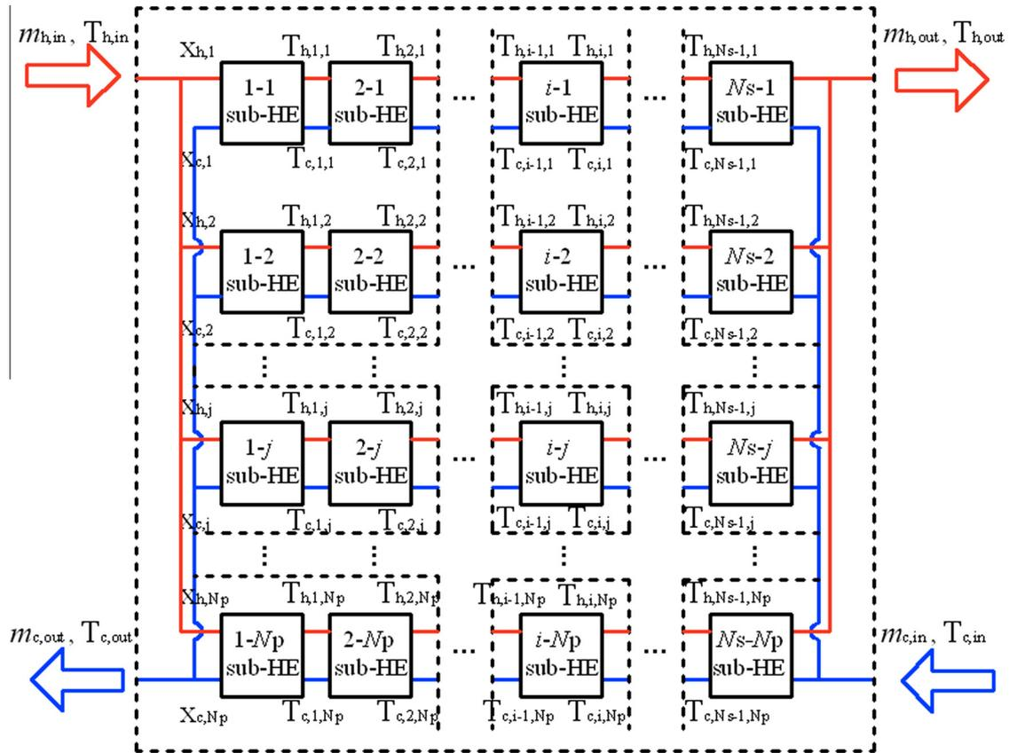
Fig. 3. The series-and-parallel arranged heat exchangers.
