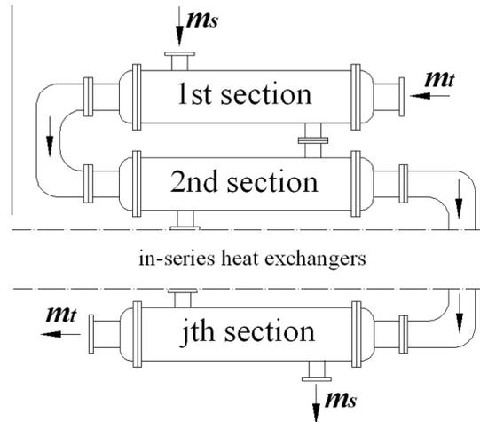
Fig. 2. The in-series shell-and-tube heat exchangers.
