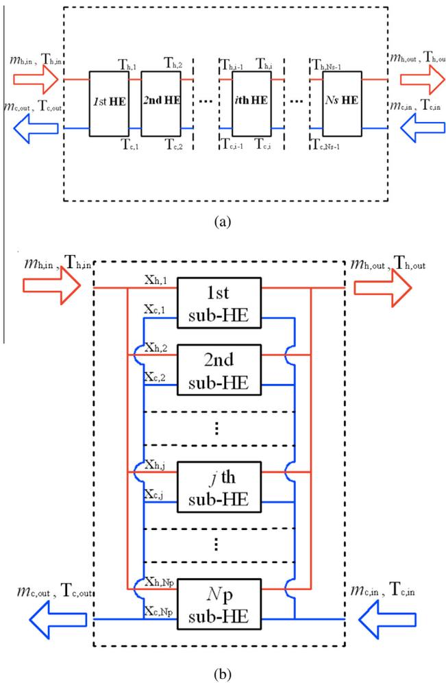
Fig. 4. The simplified heat exchangers design: (a) series-arranged heat exchanger; (b) parallel-arranged heat exchanger.
