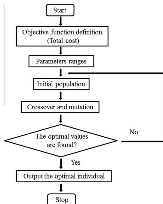
Fig. 5. Flow chart of the genetic algorithm using the total cost as objective function.
