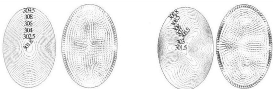
图 1 W_p = 8.87 \times 10^{-6} W 时的截面温度场和流场 Fig. 1 The temperature field and velocity field ( W_p = 8.87 \times 10^{-6} W)
