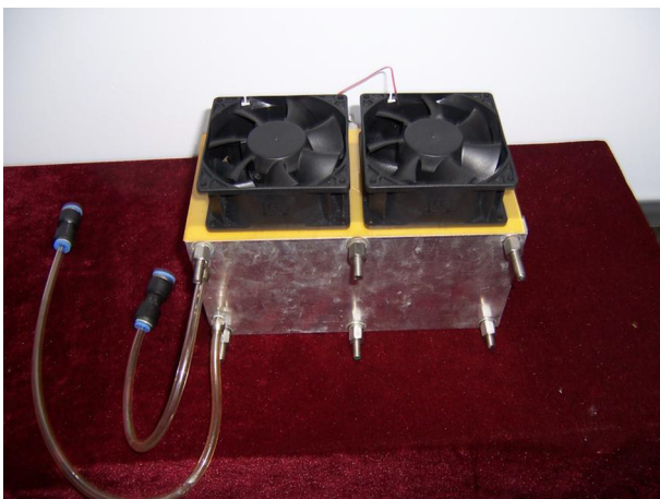
Fig. 2. Structure of the air-cooling stack.
