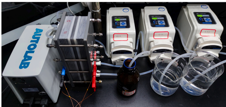
Fig. 2. Experimental system of the RED stacks.
