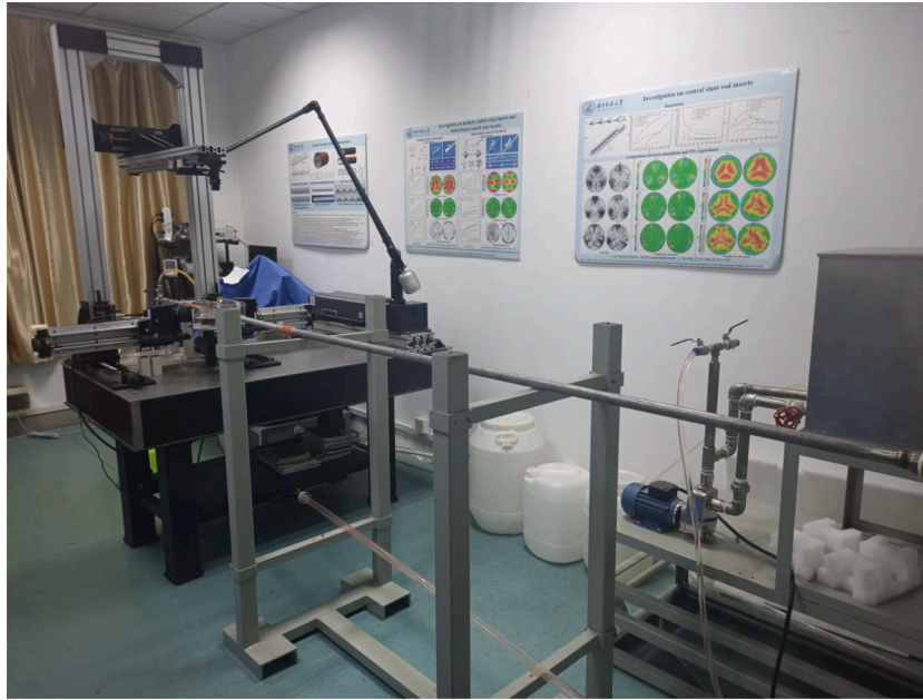
Fig. 5. The physical diagram of the Stereo-PIV system.
